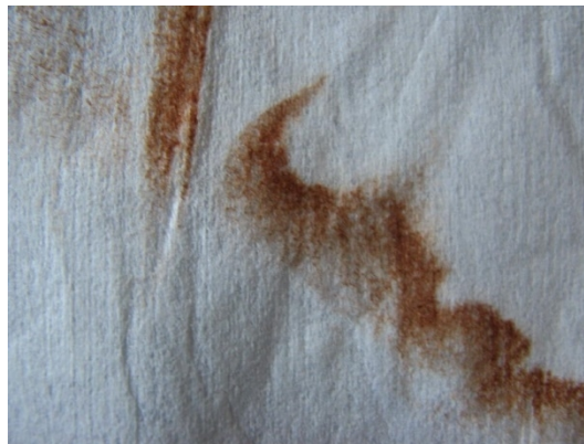
Wipe test of a production vessel
