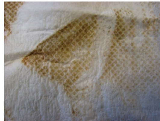
Wipe test of a WFI pipe
